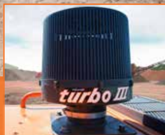
Centrifugal pre-cleaner Turbo III
