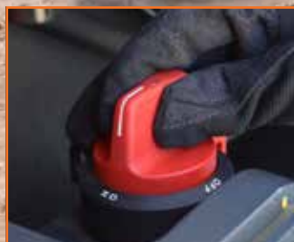
Battery cut-off switch
