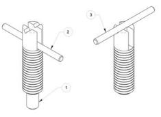
SPRING PLUNGERS 1 NOSE 2 T-HANDLE - ENGAGED 3 T-HANDLE - DISENGAGED
