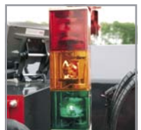
Overload warning lamps + auto stop + alarm
