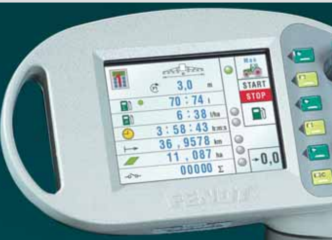
A fuel consumption display is integrated in the Varioterminale on the 800 Vario as standard. This shows the current as well as average fuel consumption and has two sum counters. Fuel consumption per hectare can also be logged at the same time in the on-board computer.
