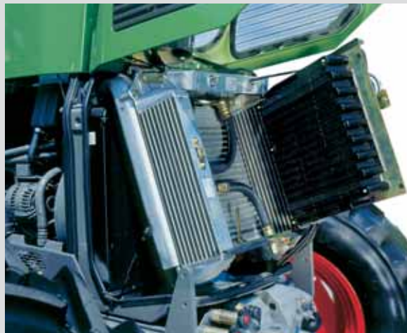
The 800 Varios have efficient cooling units with maximum service-friendliness. The cooling units for hydraulic oil, transmission oil, fuel and air-conditioning can be swung up away from the radiator to give you better access for cleaning.
